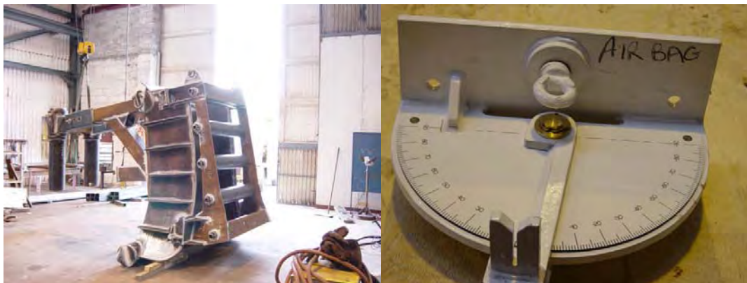
(STOLT OFFSHORE - OVERBOARD DUMP CHUTE & ALIGNMENT PROTRACTORS)
