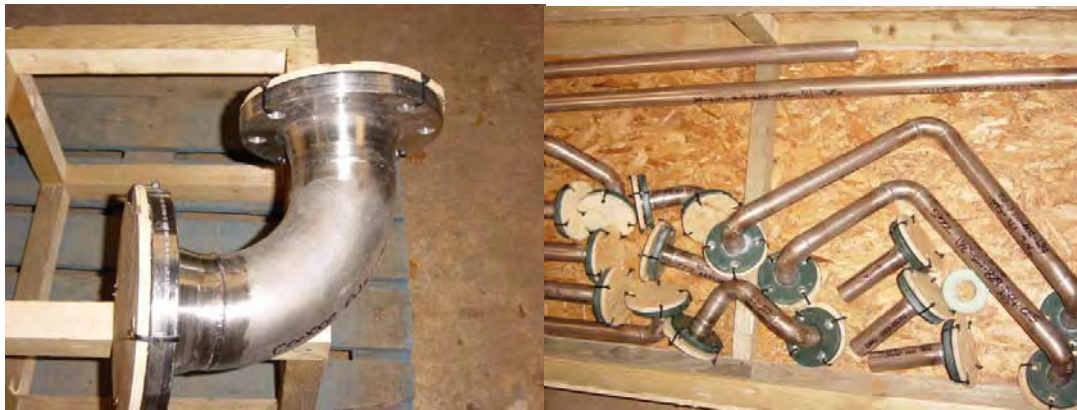
(JUDY - DUPLEX SPOOL AND NORTH ALWYN - CUNIFER SPOOLS - BEING CRATED PRIOR TO SHIPMENT)
